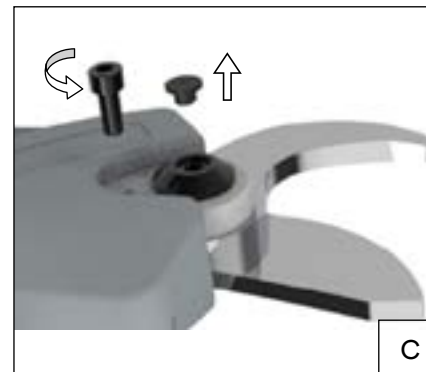
C. Remove the M5 screw by turning counterclockwise as shown in the picture, also remove the rubber cover.
